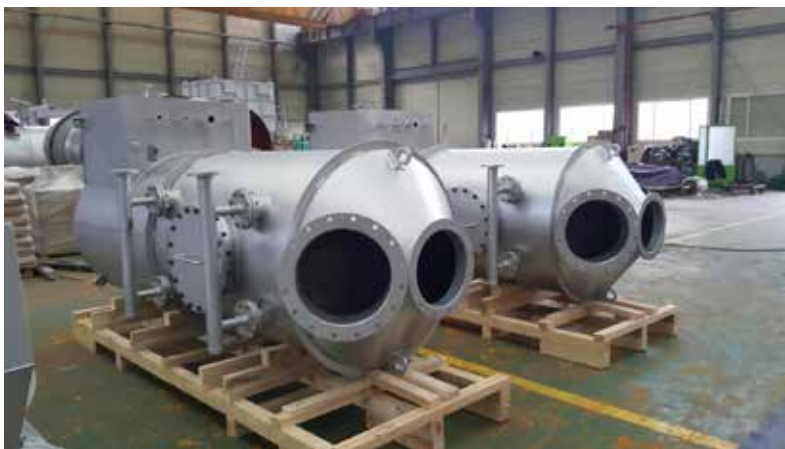
Stainless steel 304 Wet scrubber equipped with demisters, palling rings, spray nozzles, and spray pumps.
