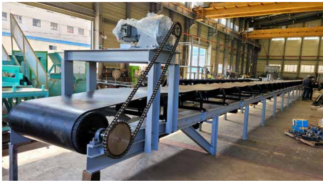
Horizontal belt conveyor, 51m installed together with 4 rotary screens and platform in apumping station, Bangkok, Thailand 2019.
