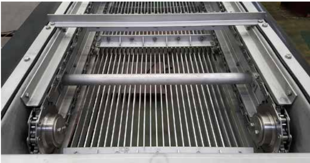
25mm bar clearance of coarse bar screens and submerged bottom sprockets made of stainless 304.
