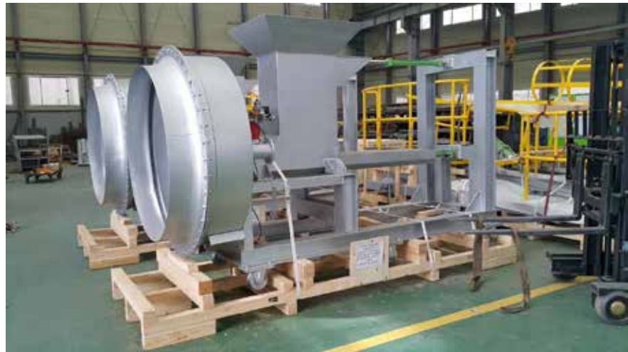
Automatic waste feeding system actuated by hydraulic power unit.
