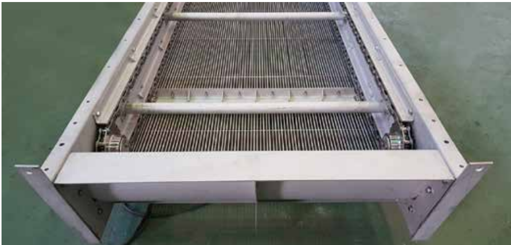
10mm bar clearance of fine bar screens with wedge bars to avoid clogging of bar space. Made of stainless steel 304 applied.
