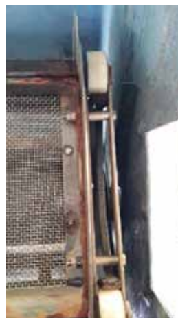
Roller chain. Roller is made of special engineering plastic.
