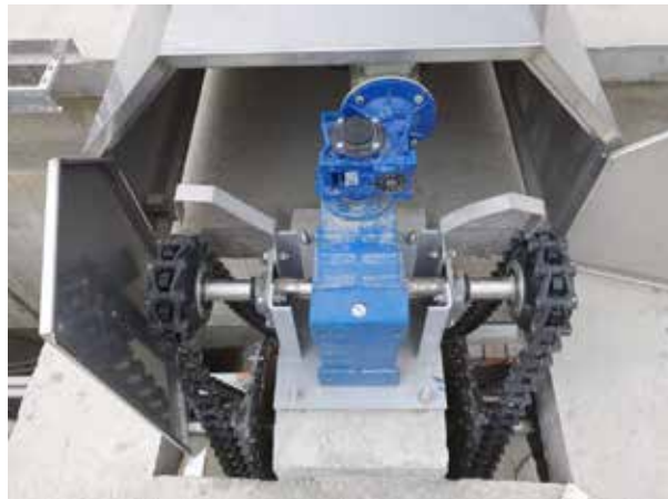
Driven sprocket, Head sprocket, Drive chain, and Drive system by helical bevel gear motor and reducer.
