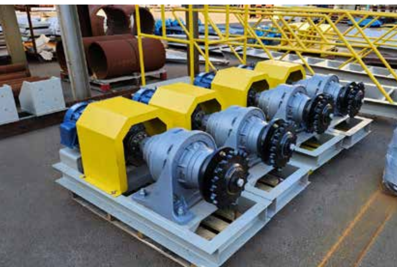
Assembly for rake, shaft, sprocket, main chain, chain tension unit & front screen.
